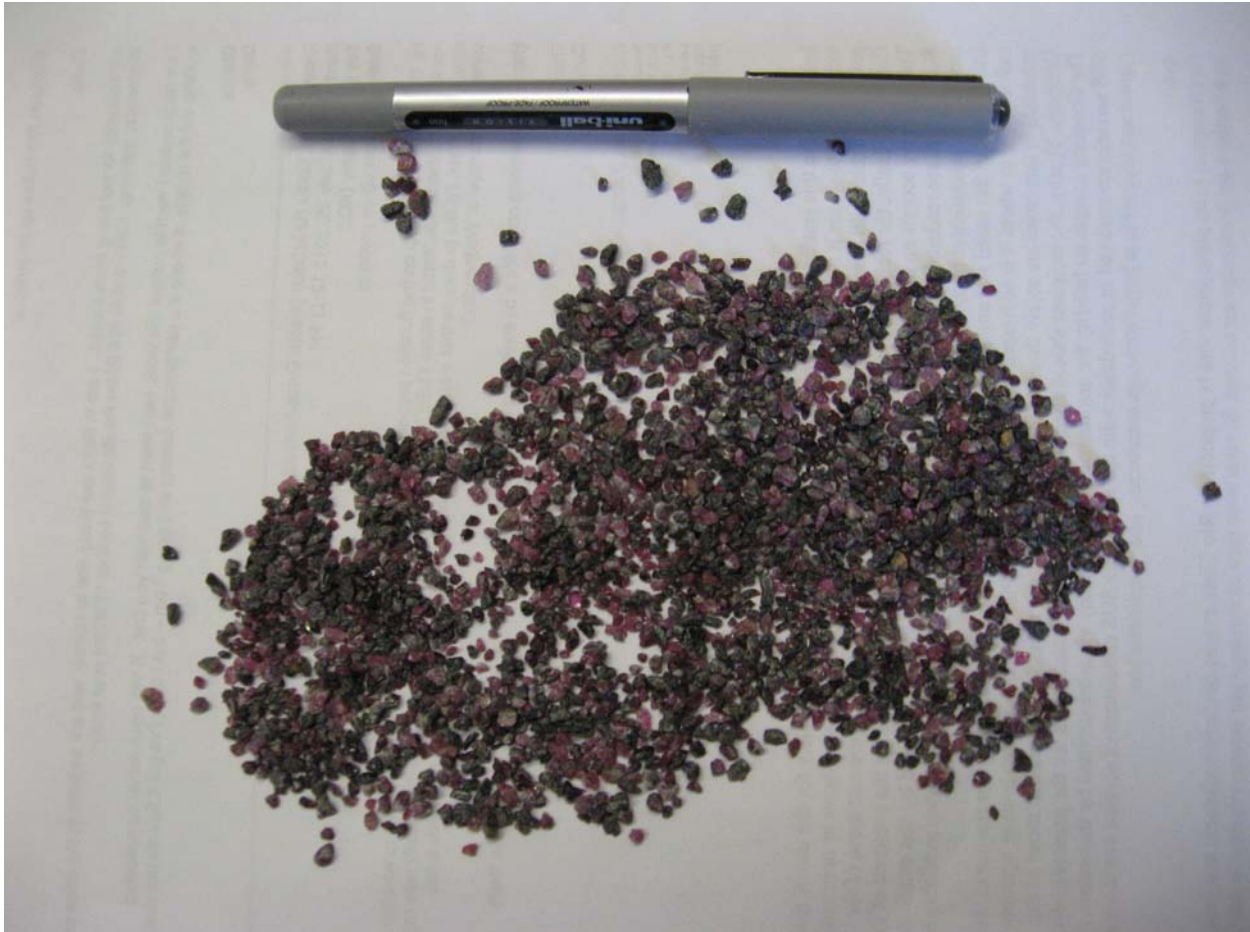
Figure 1: Material selected for test work consisting of ruby crystals and gangue silicate minerals
